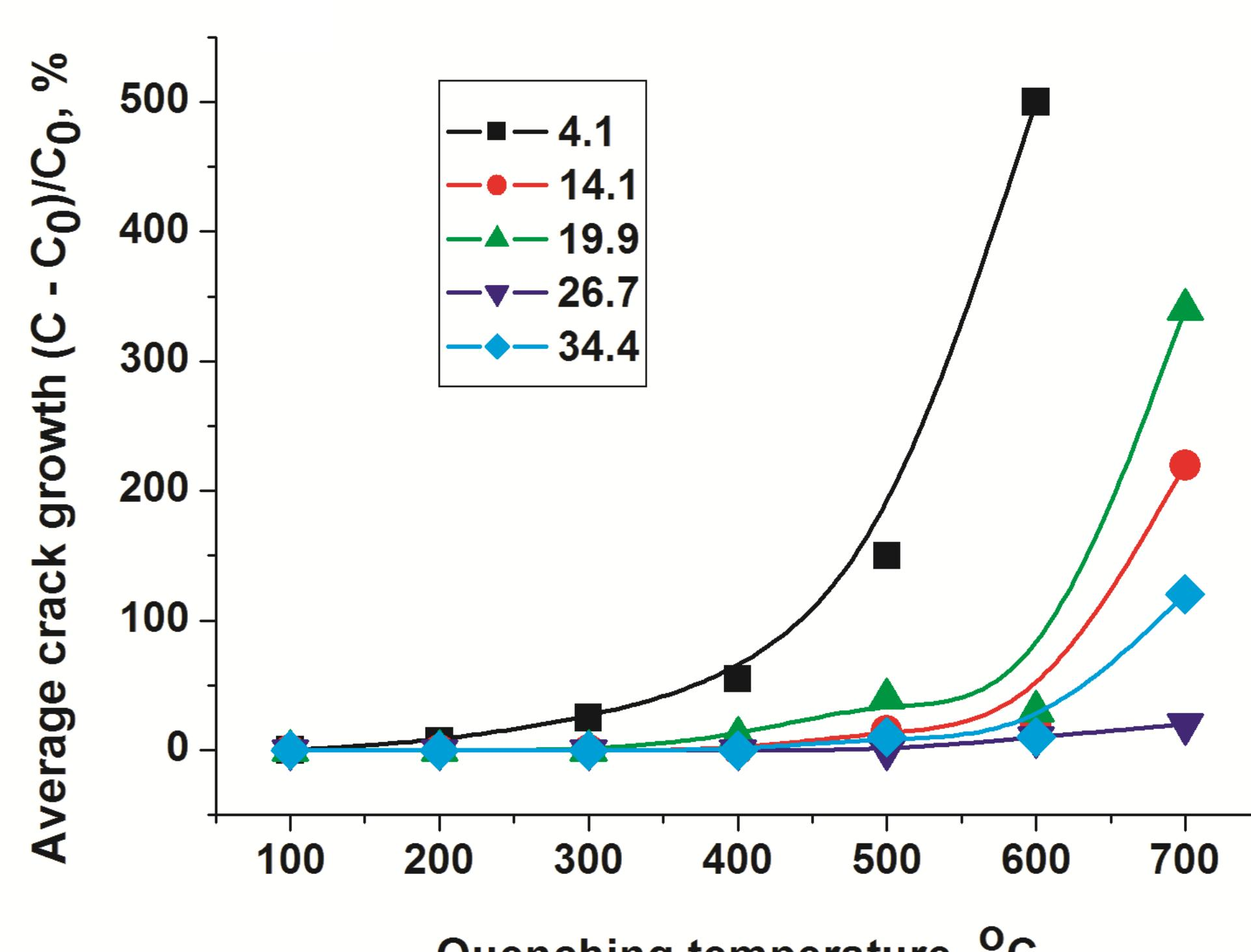
Indentation crack growth after quenching of
