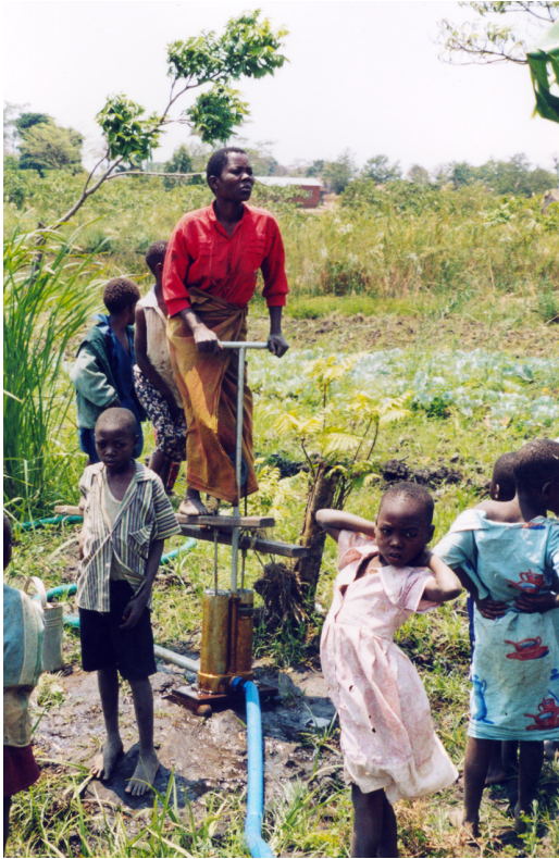
Figure 2 – Treadle pump irrigation and dambo agriculture
